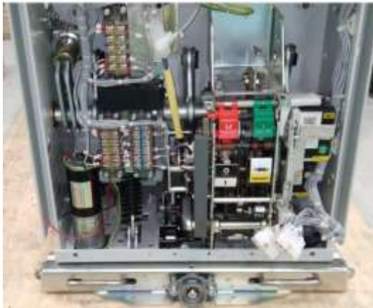
Motor truck - The racking mechanism with motor mounted on CB
